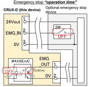
Photo-coupler permissible value: Rated VCEO:80[V], VECO:5[V], IC:30[mA]
